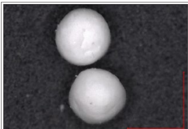
Figure 2 Morphological characteristics of self-nanoemulsifying matrix pellets
