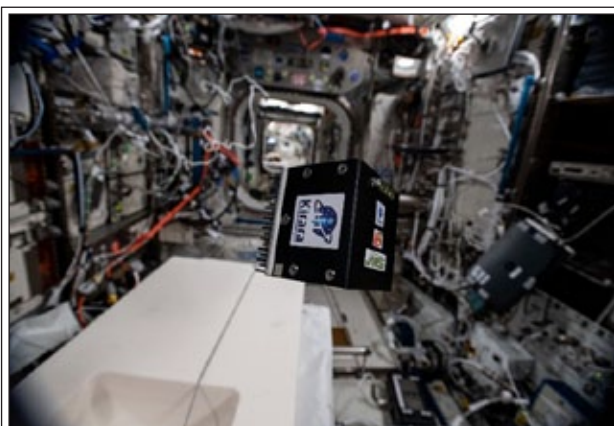
Figure 2 The "KIRARA" cube platform with samples for microgravity testing
