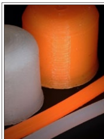
Figure 2 The PVA (white) and PLA (orange) filaments and the end-product carriers
